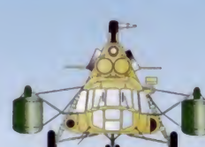
AWACS HIP: The Mi-17 was even converted to act as an airborne early warning and control machine with side-mounted radar aeriels.
